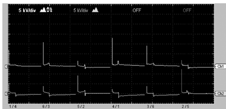
Figure 4-9 Incorrect polarity setup
